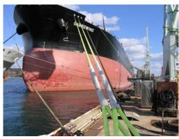
diameter of 10mm can support a weight of about 20 tons (theoretical value).
