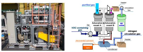
Nitrogen Cycle Desorption Method K-Filter VOC Treatment Systems (Left: Exterior view of the system. Right: Process flow)
