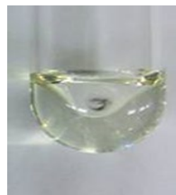
These photos show how melted PET resins, produced using TOYOBO GS Catalyst®, antimony, and titanium as catalysts from left to right, change in appearance after being exposed to heat of 300 degrees Celsius for two hours.
