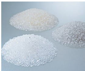
PET resins (front) produced using TOYOBO GS Catalyst® and PET resins produced with antimony catalyst (back right) and with titanium catalyst (back left).
