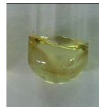
These photos show how melted PET resins, produced using TOYOBO GS Catalyst®, antimony, and titanium as catalysts from left to right, change in appearance after being exposed to heat of 300 degrees Celsius for two hours.
