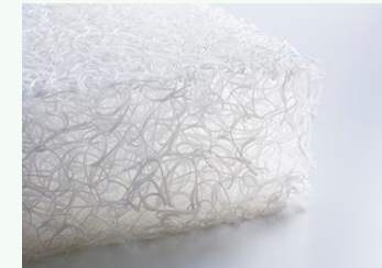
Three-dimensional cushion material "BREATHAIR" Materials that have rubber elasticity and formed with a unique steric structure
