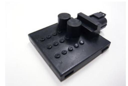
Example of sealing on an electronic component
