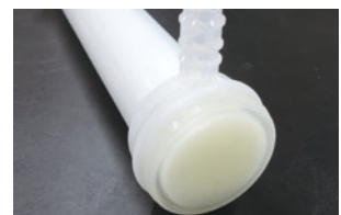
Dialyzer for artificial kidney using a hollow fiber membrane
