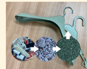
Upcycled apparel products (hangers made from crushed and pelletized fiber scrap)
