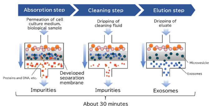
With the three steps of absorption, cleaning and elution, purified exosomes can be recovered
